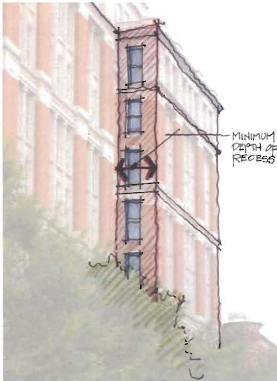
Facade recesses should have a minimum depth to allow windows to be placed in the face perpendicular to the street.
