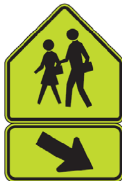
Figure 7. School Crossing Assembly, Located at Crossing (S1-1 and W16-9p)
