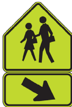
Figure 3. School Crossing Assembly, Located at Crossing (S1-1 and W16-9p)
