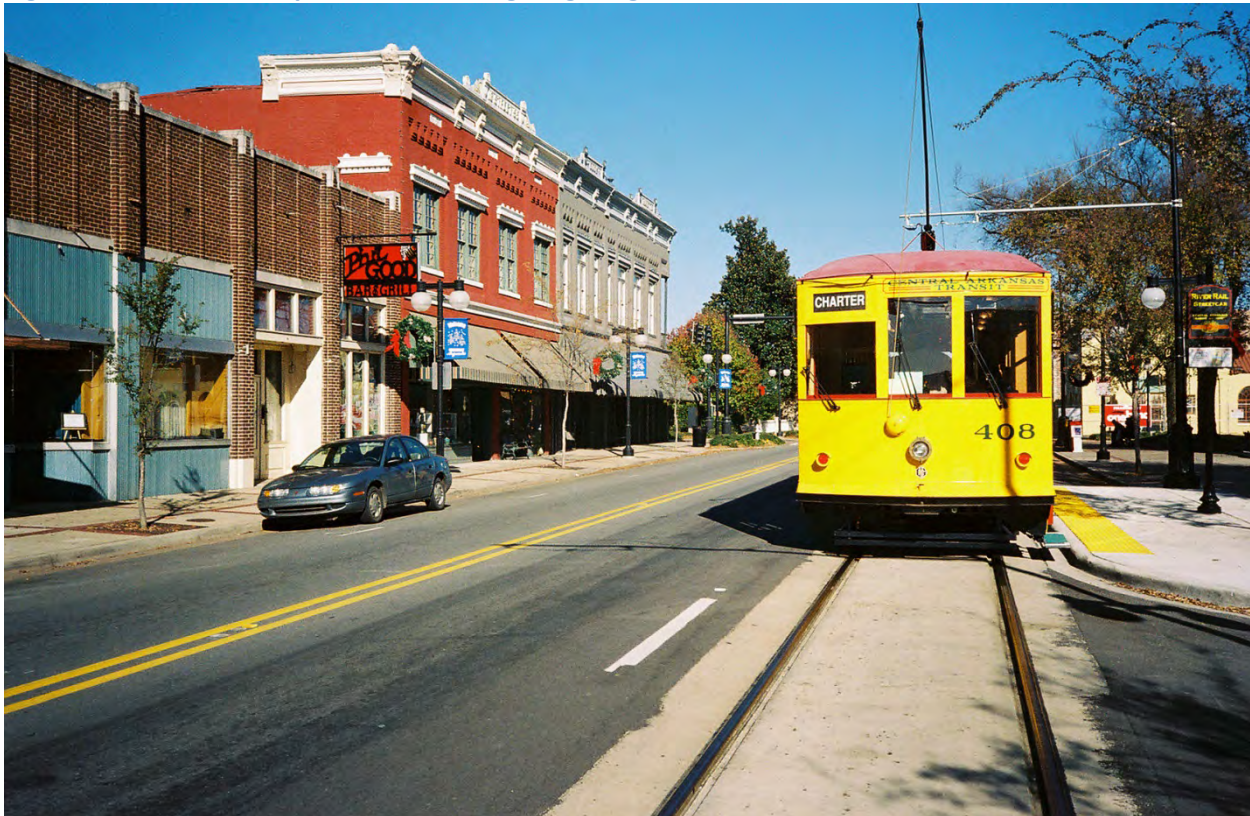
Figure 8. Sidewalk Bump-out for Boarding/Alighting; Little Rock, Arkansas
