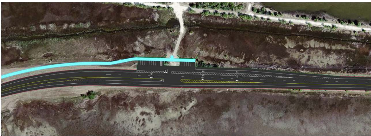
Figure 6 Recommended Turn Lanes at McQueen's Island Trailhead Entrance
