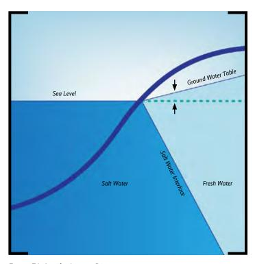
Figure 7.1-Aquifer Impact Diagram
