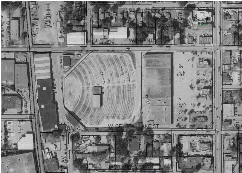
An example of form-based codes that require building placement against the street. In this redevelopment site in Orlando, Florida, the placement of new buildings against a network of streets being added to the block defines the street space and makes future widening difficult, if not completely impractical. This is an appropriate street treatment for an urban context.
