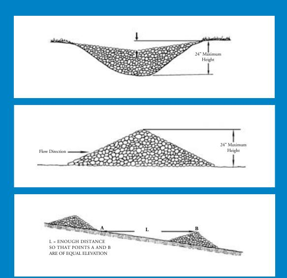
To stop concentrated flows on slopes that drain 5 acres or less, install a series of rock check dams. Place graded, size 2- to 10-inch stone the entire width of a ditch or drainageway so that the center is lower than the edges. (See middle diagram.) Stone piles should not exceed 24 inches in height. A series of check dams should be spaced apart so that the toe of the uphill dam is at the same elevation as the top of the downhill dam. Do not install check dams in streams.
