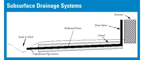
If the site does not allow for regrading or installing diversions; or if surface depressions, a high water table, or hydric soils are present; an underground drainage pipe may be necessary. Pipe grades should be gentle enough to allow water to enter but provide enough fall to drain readily. The water should empty into an existing drainage ditch or curb inlet where possible.
