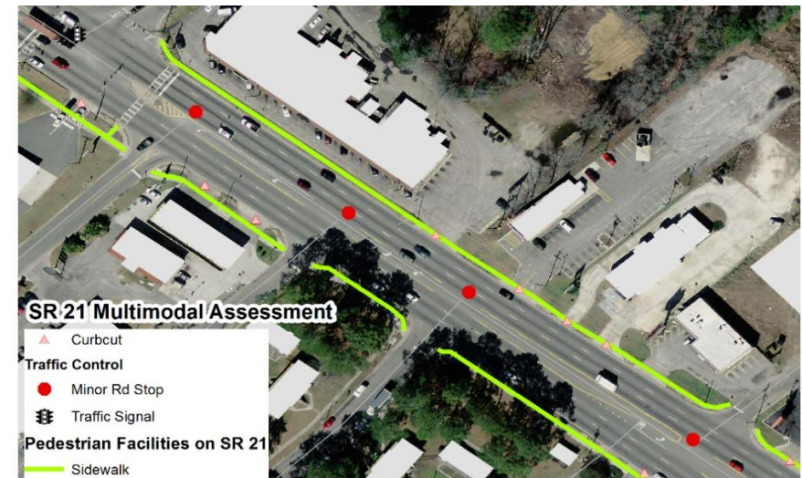
Figure 4-19: Example of Inadequate Intersection Spacing on SR 21 from St Joseph Ave north to Brampton Road
