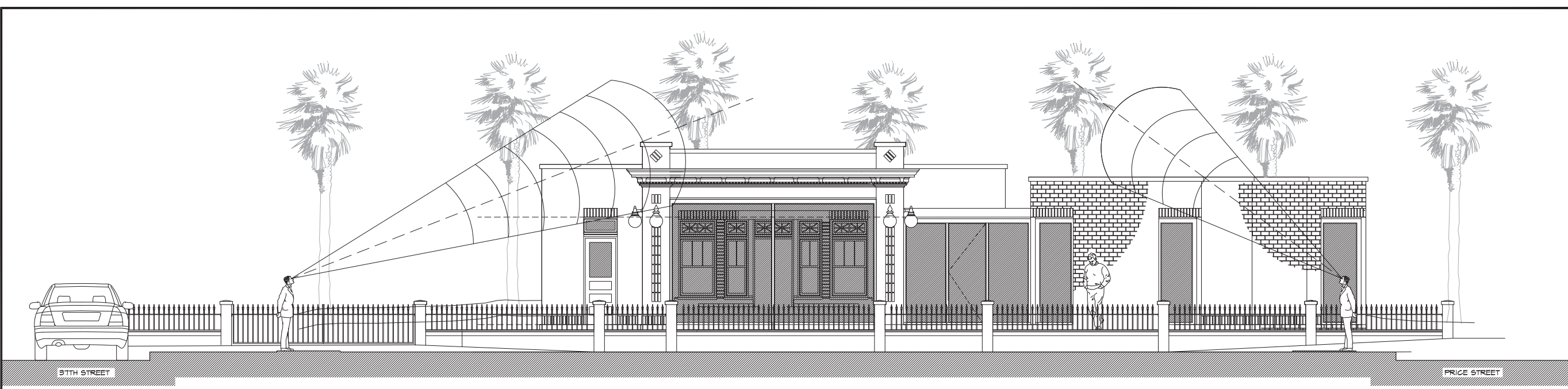
3 LINE OF SIGHT DIAGRAM SCALE: 1/4"=1'-0"
