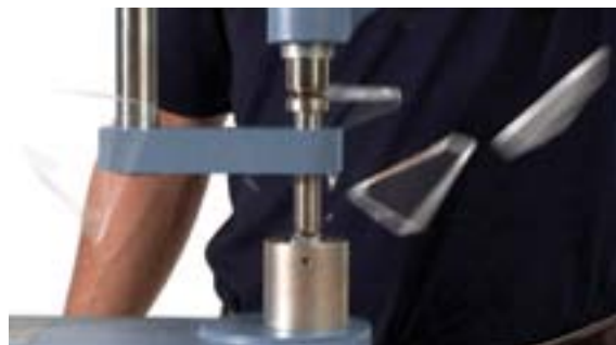
GLASS FAILS AN IMPACT TEST USING STEEL DART WITH ONE INCH DIAMETER TIP
