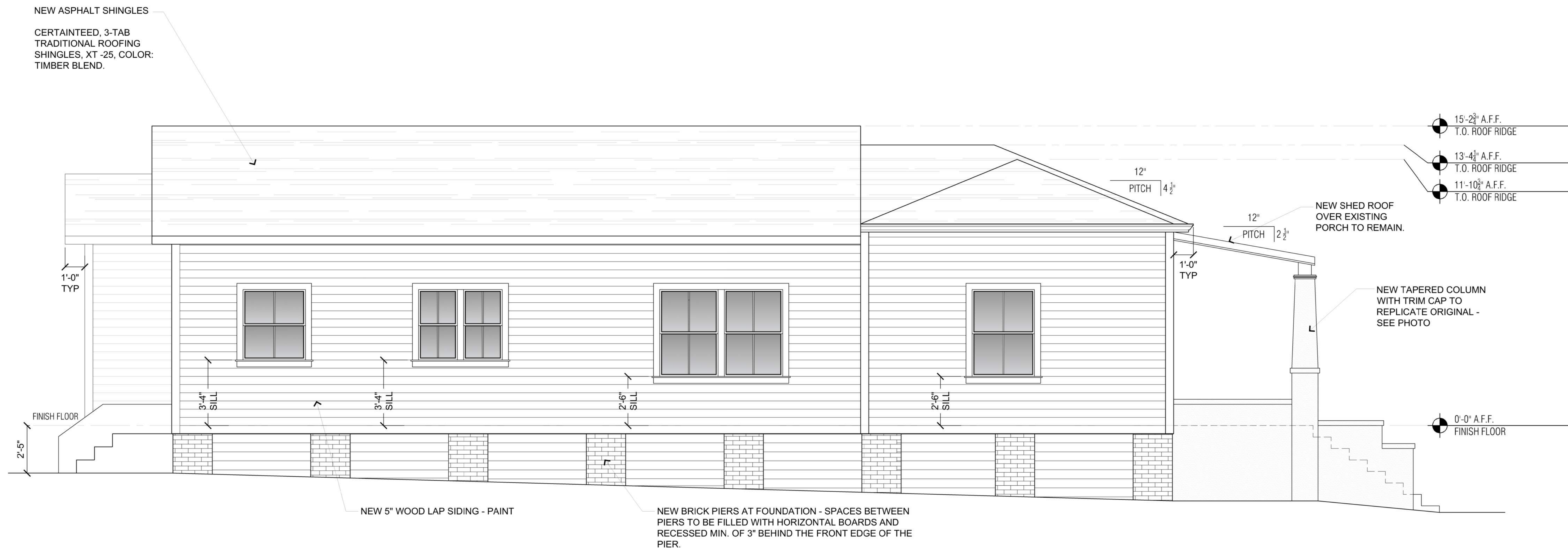
EXTERIOR ELEVATION - WEST ② 3/8" = 1'-0"
