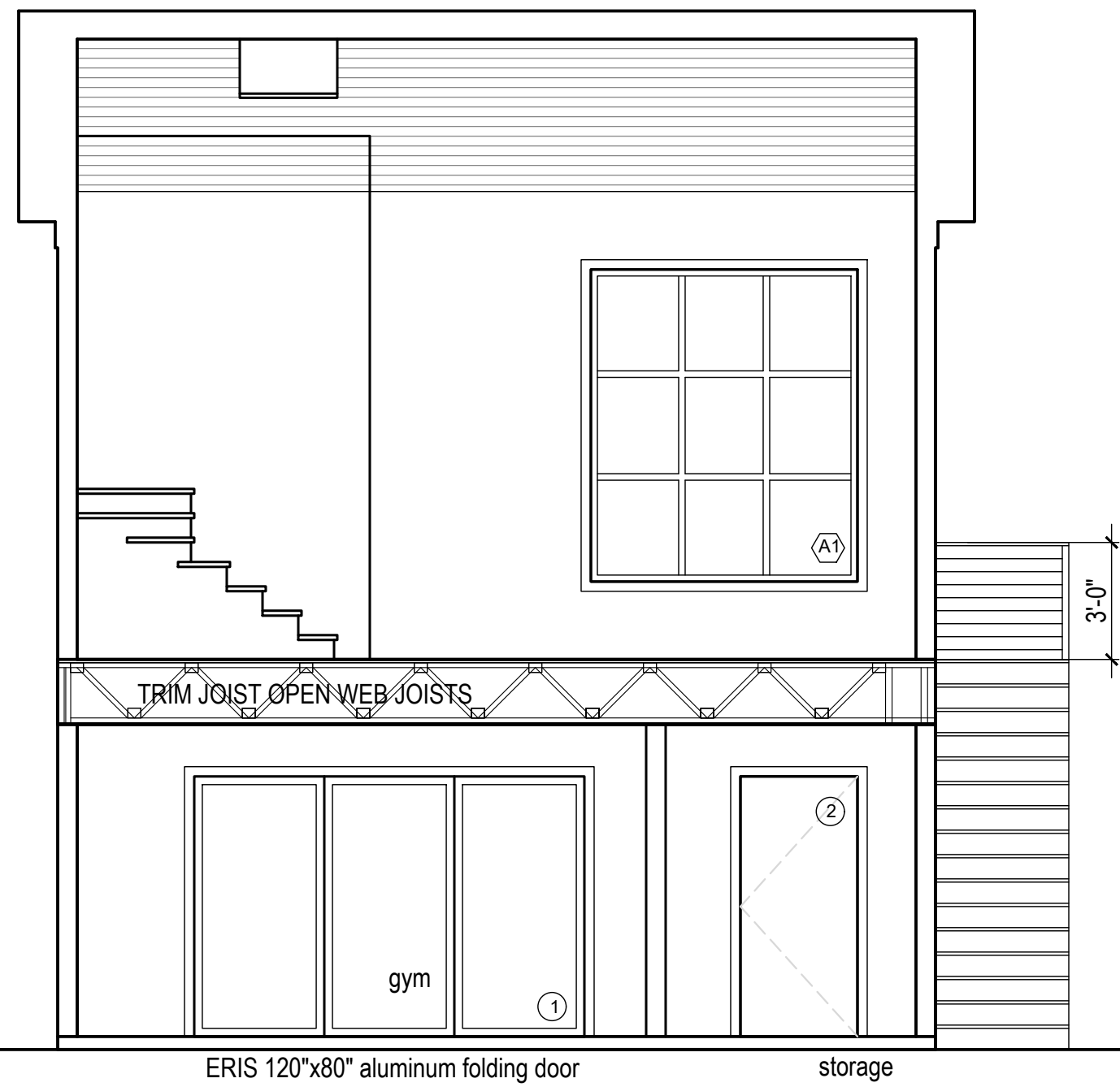
1 BUILDING SECTION LOOKING NORTH (FACING HOUSE) SCALE: 1/4" = 1'-0"
