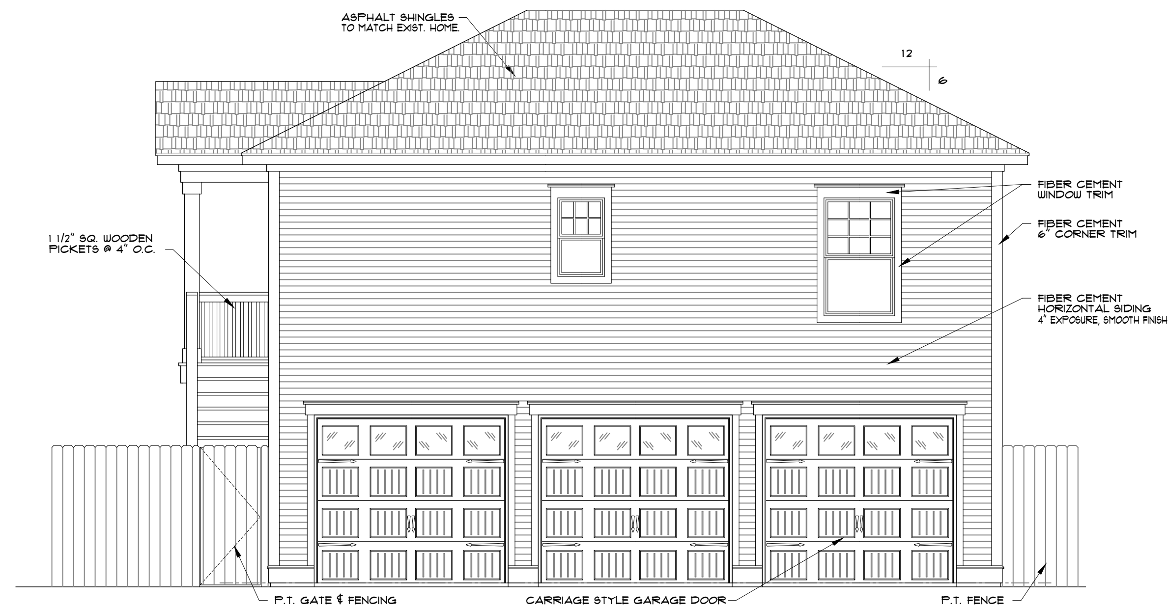
SOUTH ELEVATION SCALE: 1/4" = 1'-0"
