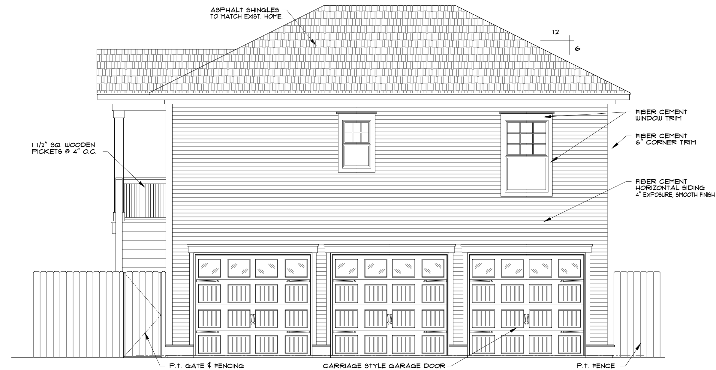
SOUTH ELEVATION - PROPOSED SCALE: 1/4" = 1'-0"
