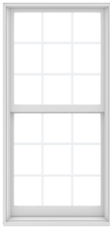
DOUBLE HUNG SEE ELEVATIONS
