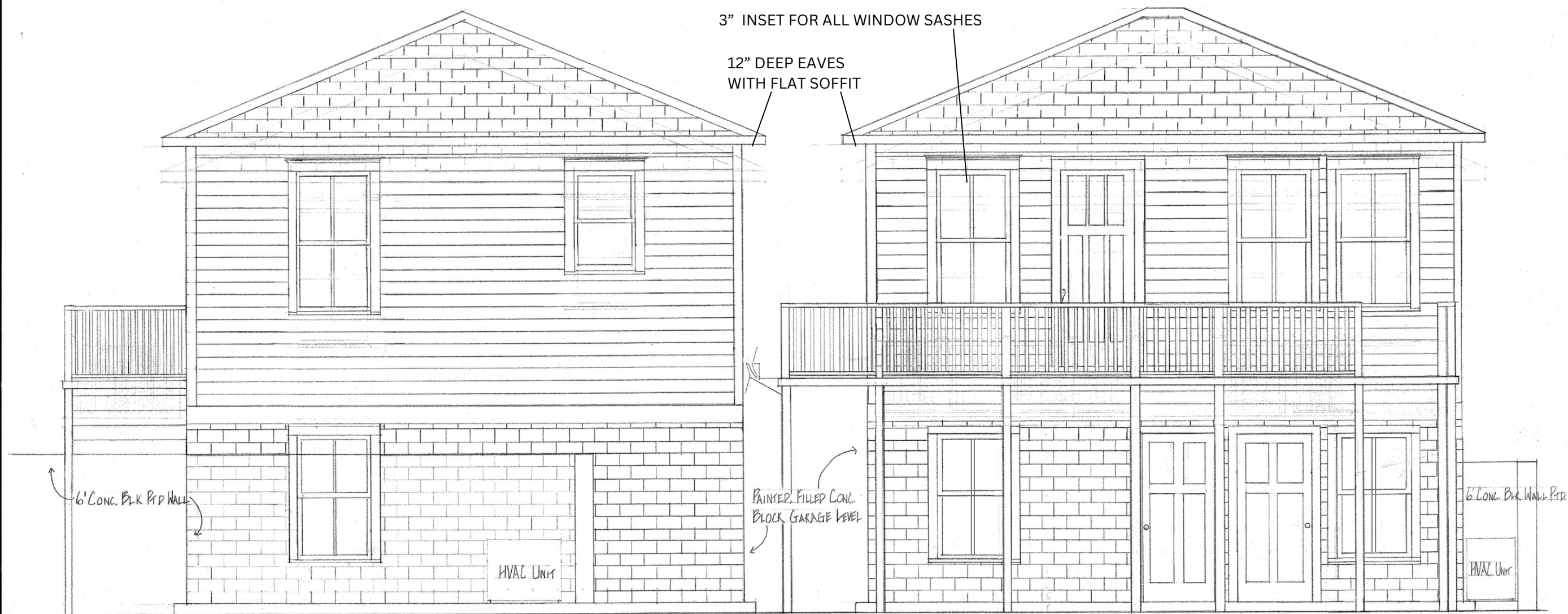
EXTERIOR ELEVATION WEST FACE
