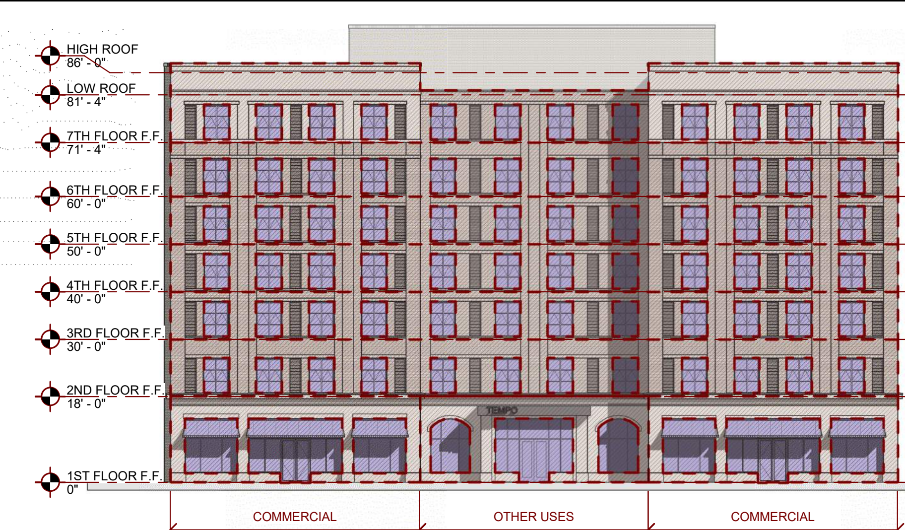
12 HD BR 0.5 WINDOWS AND DOORS - EAST (BRYAN STREET) ELEVATION 1" = 20'-0"
