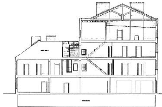
These recent architectural drawings of the still-standing City Hotel building indicate the differences in its four-story Bay Street facade (left below) and its three-story rear which faces Bay Lane (right below). Drawings by Brito & Stembridge, Inc., Savannah, reproduced with permission of Corim, Inc.
