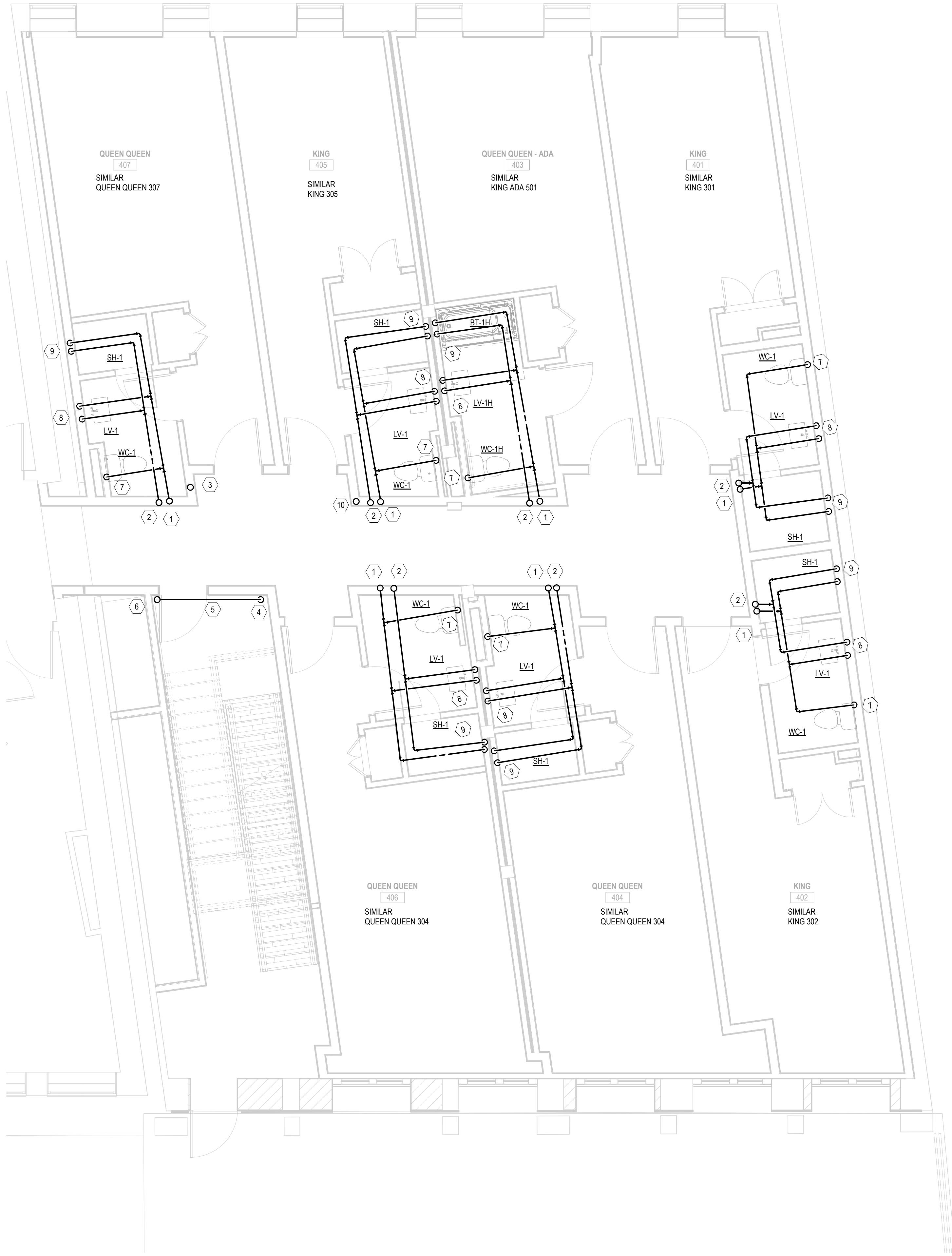
1 Overall-Plumbing Plan-04-DOM Water P1.24 1/4" = 1'-0"
