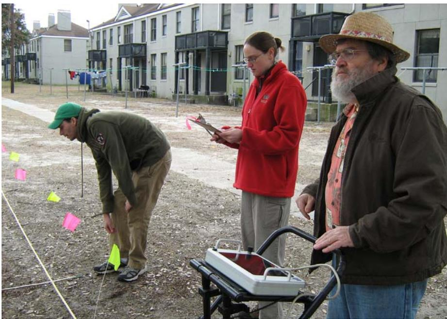
Figure 42. Collecting GPR data in the greenspace between Yamacraw Village apartments.
