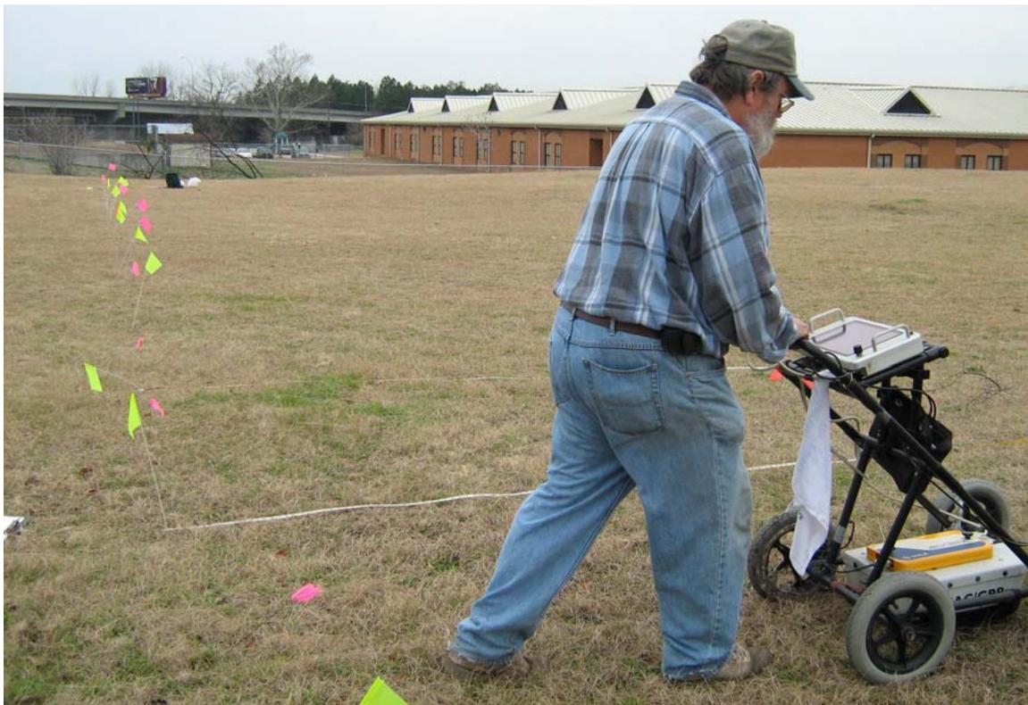
Figure 132. GPR Survey on Morgan and Boykin tracts. Note the extreme elevation differences by the school and interstate highway in the background.
