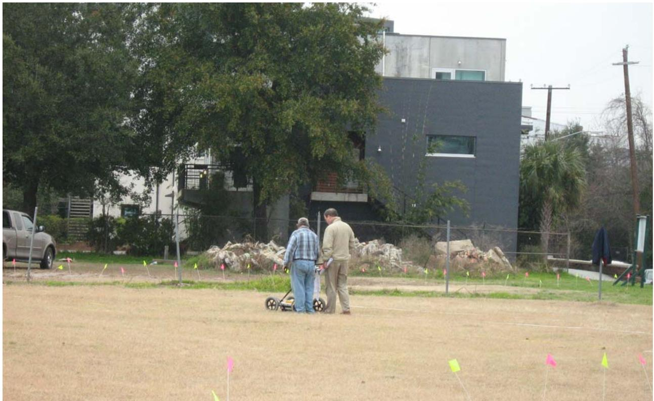
Figure 127. GPR survey on Morgan and Boykin tracts in the Jewish Cemetery area. Note the rubble pile in the background.
